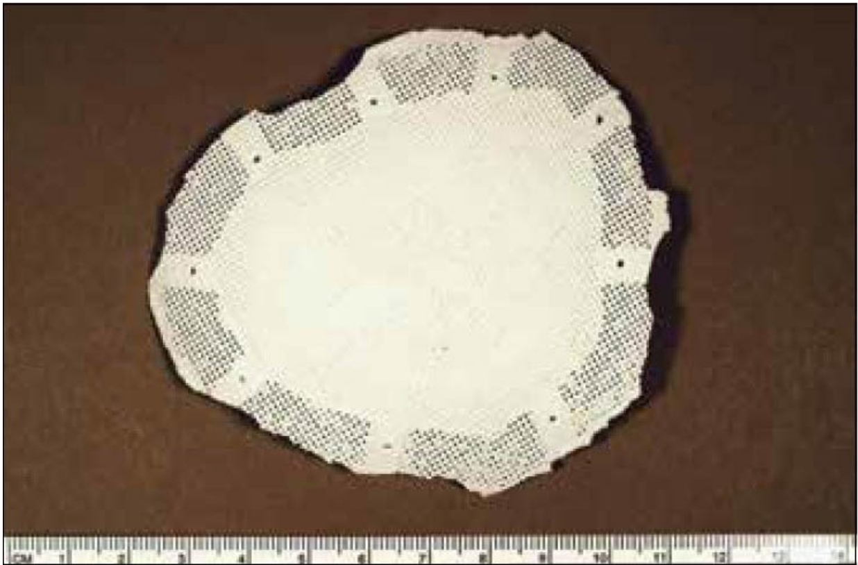
Porous resin and hydroxyapatite implant manufactured by stereolithography
