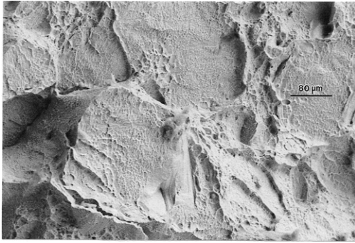
Fig. 20 – Field emission SEM images showing fracture surface features for SLM manufactured (horizontal) cylinder corresponding to elongation of 4.4%.
